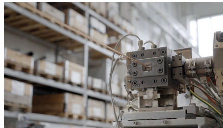
High-precision extrusion die specifically developed for hairpin production.
