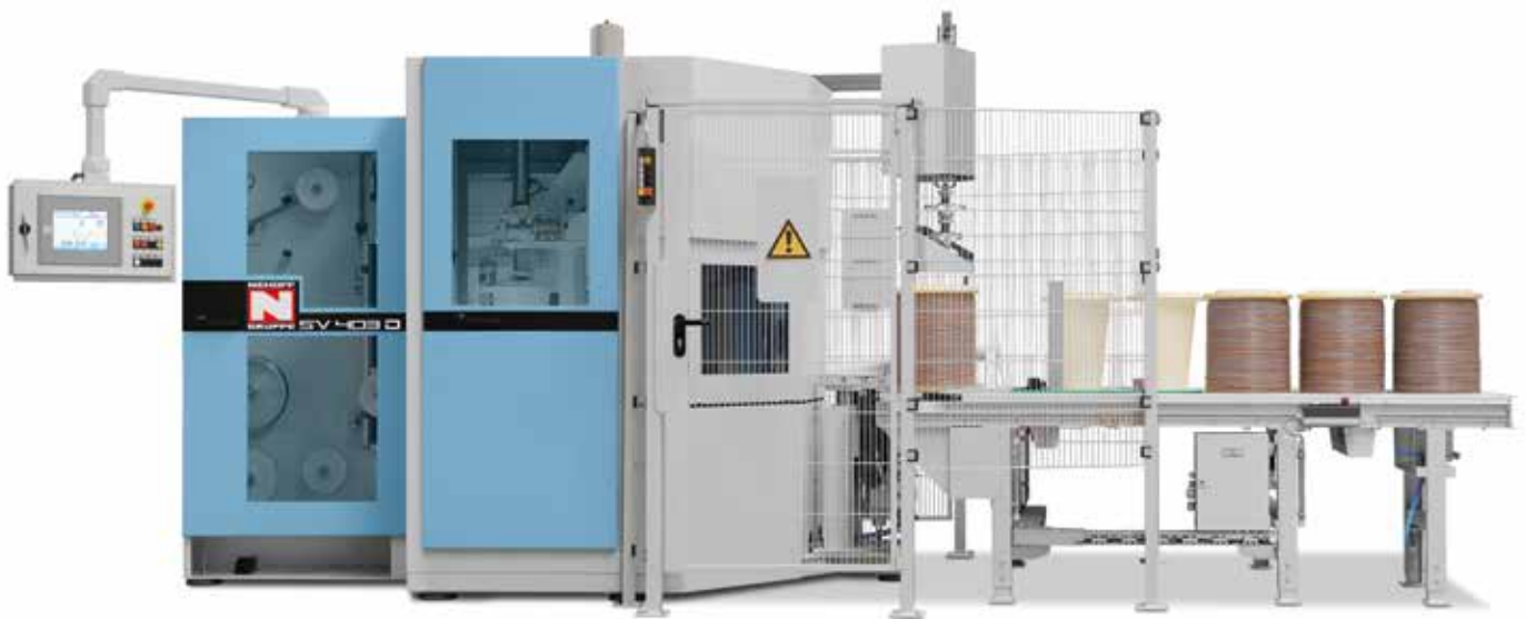
Fig. 1. Niehoff's completely automated NPS double spooler type SV 403 D.
