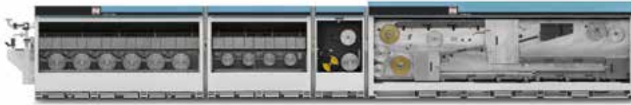
Fig. Niehoff's new MSM 88 + R 503 rod breakdown (RBD) line using the HEAT system.
