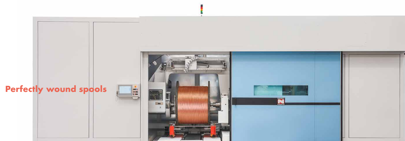
The D 2002 type double twist stranding machine is the largest model of Niehoff's D series.
