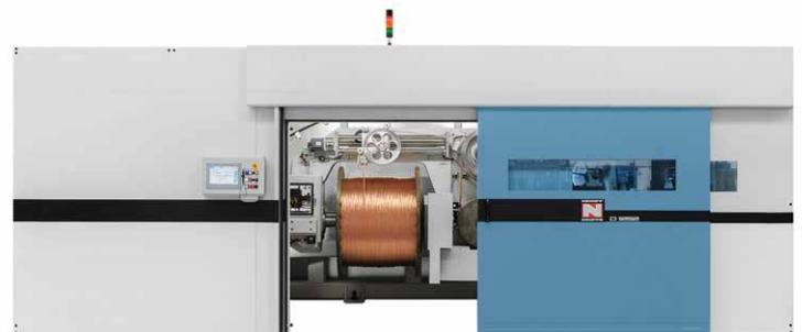
Fig. 2. Detail of a D 1252 type double-twist strander
