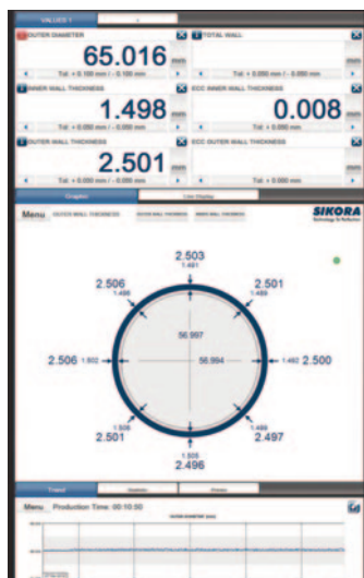
Basic visualisation at the ECOCONTROL 6000 with eight measured values
