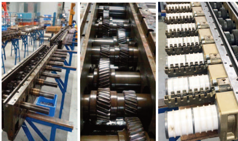
Left and centre, the gearbox of an MMH-type multiwire drawing machine with approximately 60,000 hours of operation is prepared for reconditioning. Right, the reconditioned unit.
