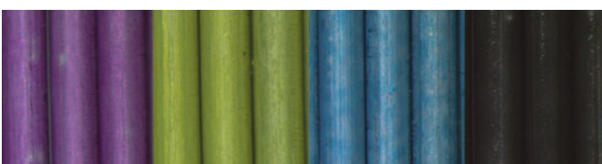
Fig 6 : Coloured hybrid polymer coated spring wire
